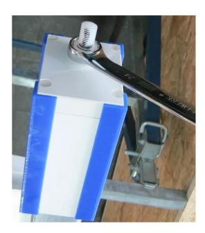
5) Insert the antenna pipe into the hollow shaft of the stand slide and fasten the fixing screws carefully at both sides
