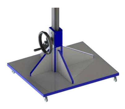
7) For changing the polarisation of the stand, pull out the polarisation pin and turn the antenna pipe by 90°. There are two hard stops for vertical and horizontal position.
