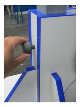
2) If the mast tube is divided, join together the divided stand tubes, and fix it with the plastic screws. Take care of the marking!
