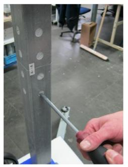
3) Install the stand slide into the stand tube
